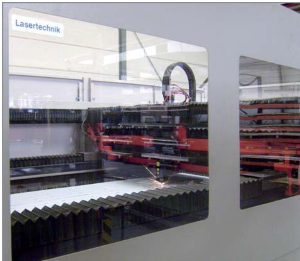
Bellows in operation
