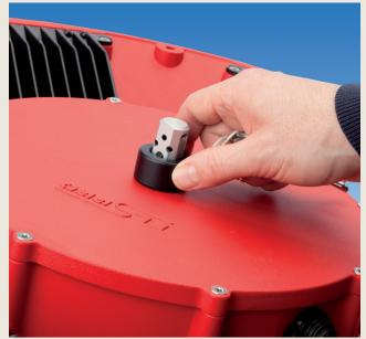
Pass the cable through the opening with the recess - Attach the angle coupling to the connector - Place the strain relief ball in the recess - DONE.
